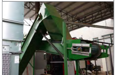
Detail of the conveyor between the chipper and the woodchip yard
