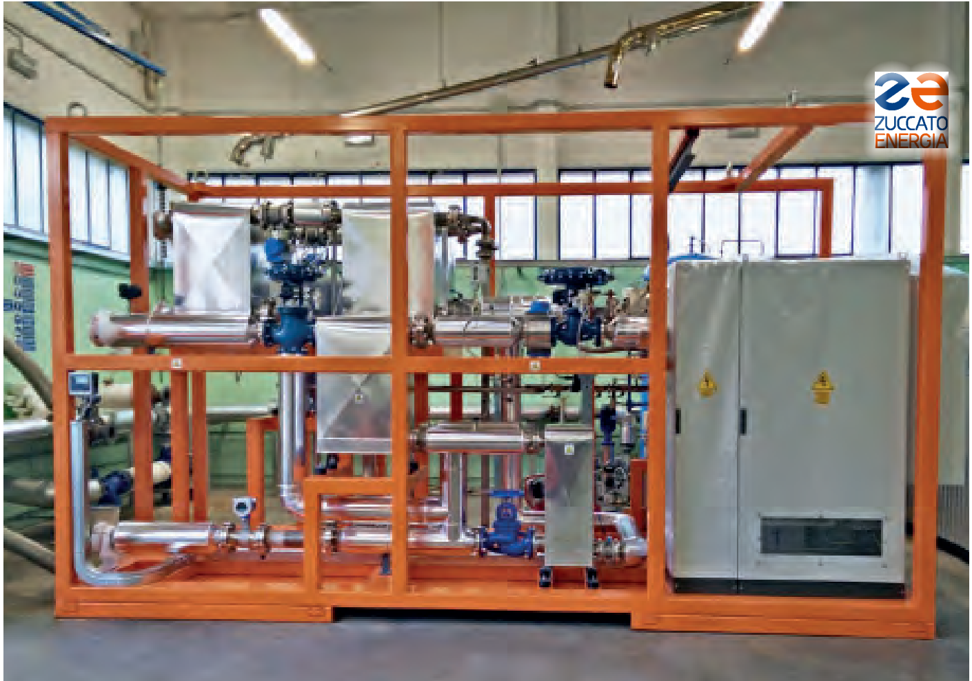
Sicilia 01 / Ragusa : The ORC system being tested in Zuccato Energia's Test Area
