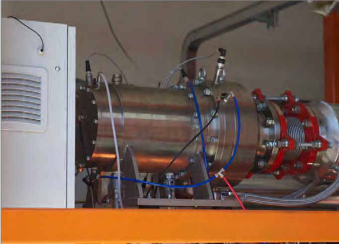
The 150 kWE turbine of the ZE-150-LT system.
